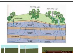
Ideally, the GSAP VMP should be sited in a well-drained location typically with sub-soils that are sandy; in such a case the digester can be placed totally in the ground. Most locations are not ideal and so the installer must place the digester as a depth such that is will never be below the water table, even during the rainy or wet season.
